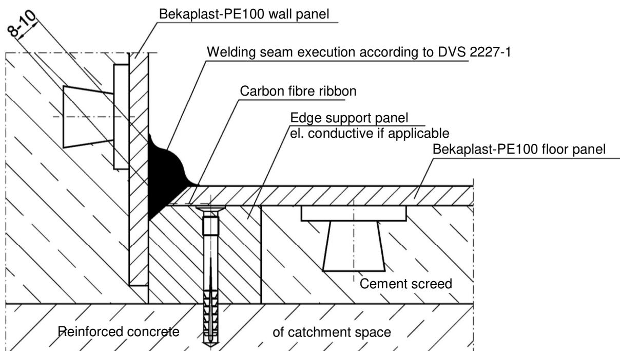
Measurements in mm
