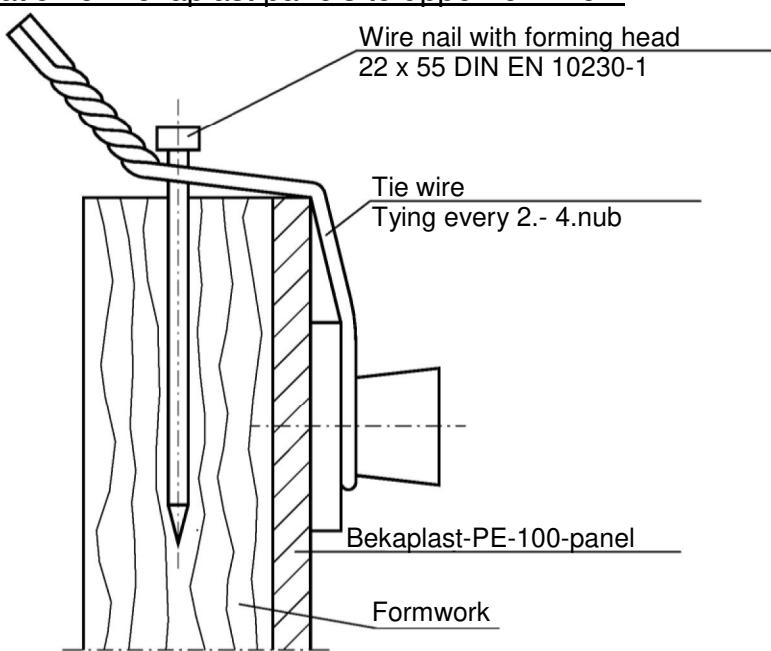
Measurements in mm
