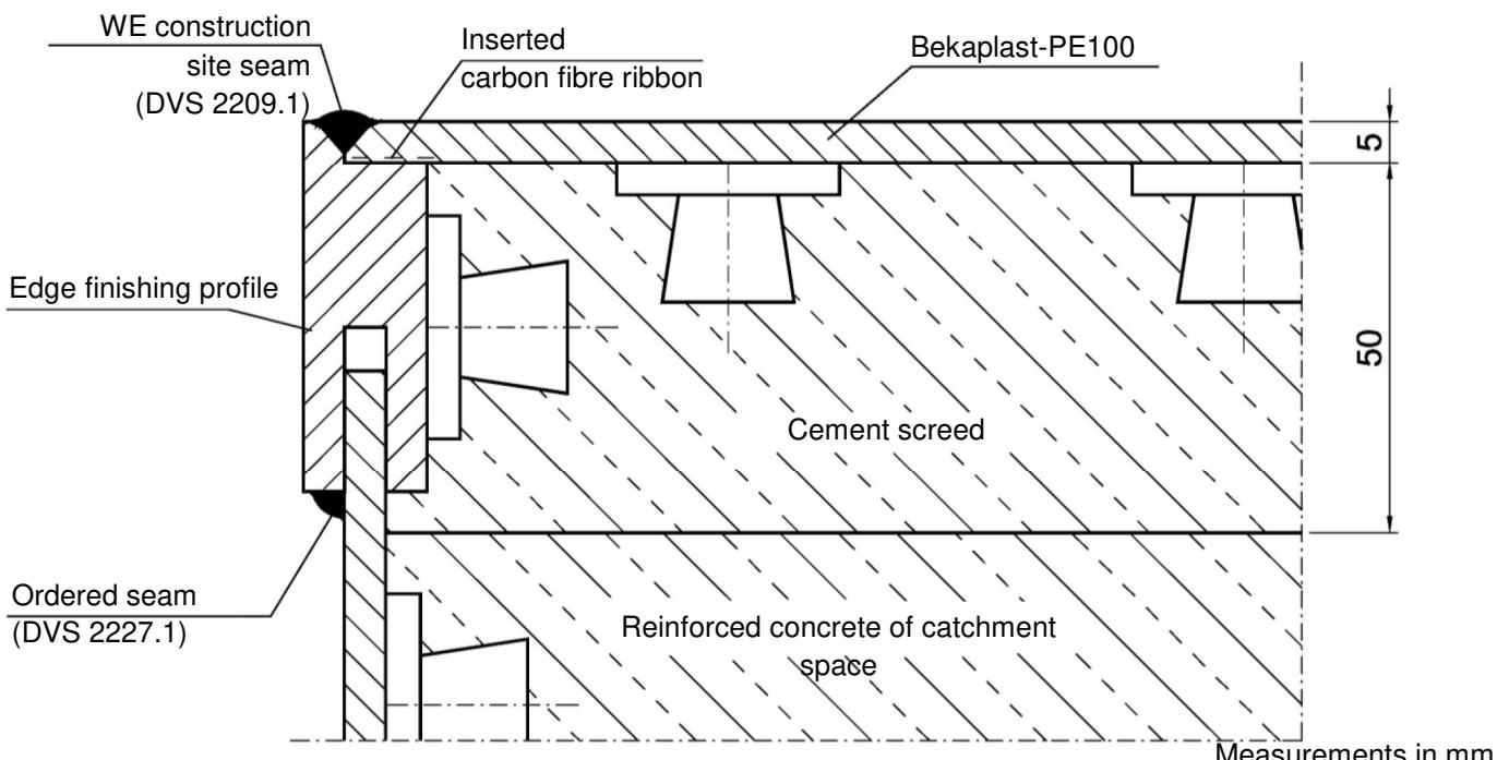
Sealing system "Bekaplast PE100" made of concrete protection slabs for the use in collection trays and rooms in facilities for the storage of materials hazardous for water
