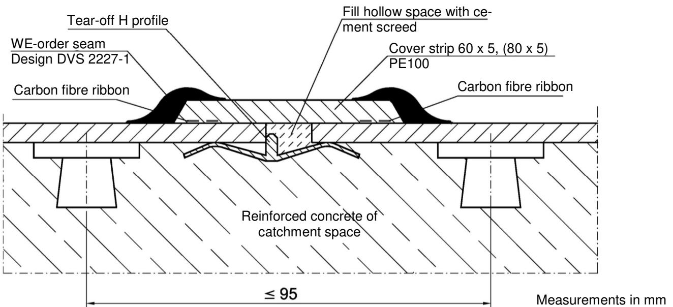
Sealing system "Bekaplast PE100" made of concrete protection slabs for the use in collection trays and rooms in facilities for the storage of materials hazardous for water
