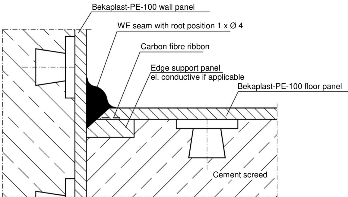
Sealing system "Bekaplast PE100" made of concrete protection slabs for the use in collection trays and rooms in facilities for the storage of materials hazardous for water
