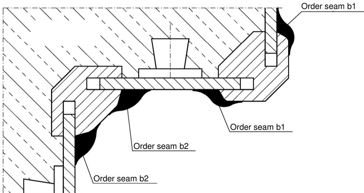
Sealing system "Bekaplast PE100" made of concrete protection slabs for the use in collection trays and rooms in facilities for the storage of materials hazardous for water
