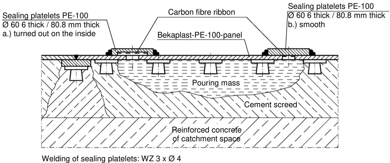
Measurements in mm
