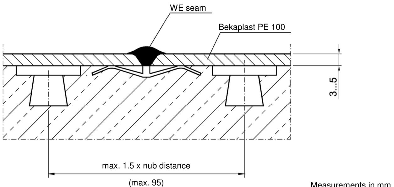
Sealing system "Bekaplast PE100" made of concrete protection slabs for the use in collection trays and rooms in facilities for the storage of materials hazardous for water
