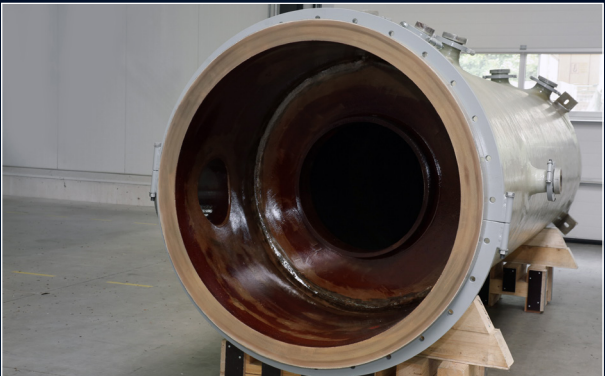
Complete HCl absorber made from KERA® Plast L / GRP for extreme operating environments. In this case, 32 % hydrochloric acid (HCl), operating temperatures of up to 120 °C, designed for an operating pressure of -1.0 / + 0.5 bar.
