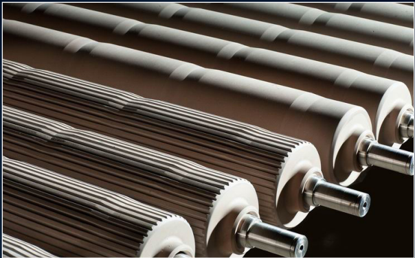
Rollers made from KERA® Complex used for cellulose processing, with 20 % sulphuric acid (H 2 SO 4 ) as the process medium and a working temperature of 70 °C.
