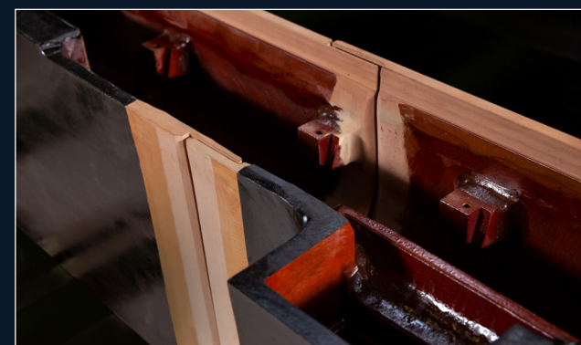
Sulphuric acid process vessel made from KERA® Plast XL in the viscose fibre industry. The many individual segments are precisely assembled and securely bonded together on site.
