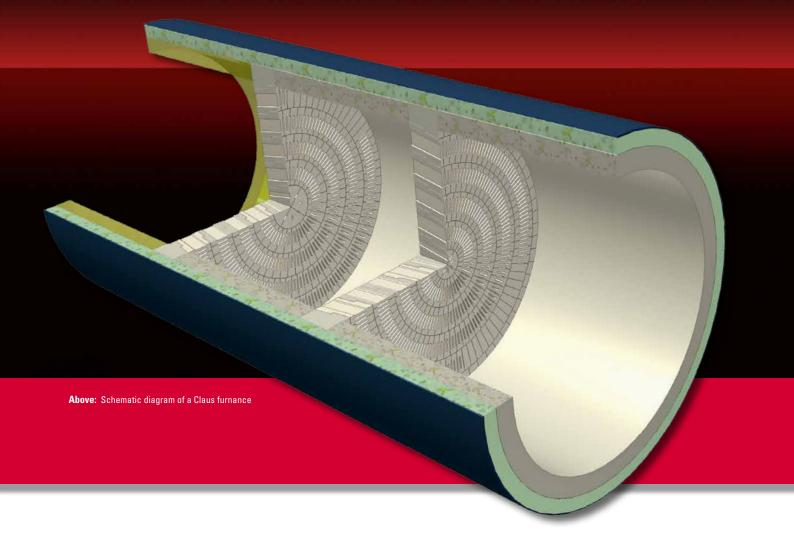
For the chemical industry, STEULER-KCH supplies products for thermal processing units, treatment plants, incinerators and waste disposal facilities. Depending on the specific loading conditions, the appropriate lining materials are used in rotary tube furnaces and in sulphur and thermal oxidation units for residual liquids and gases. Qualities based on bauxite, andalusite, chromium-andalusite, corundum or chromium-corundum serve as wear materials.
