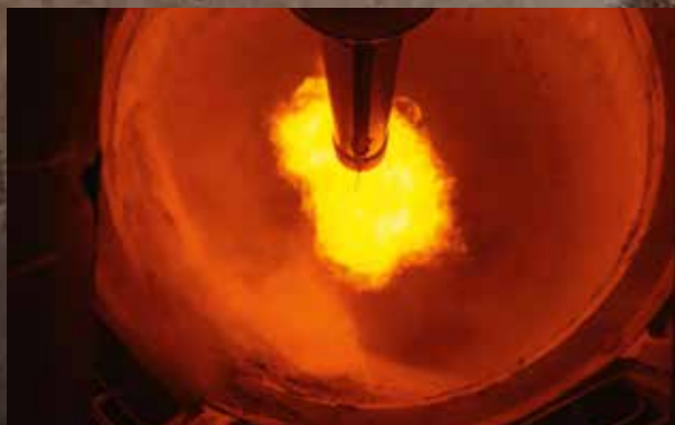
Ignition and heating-up of a newly lined lime kiln.
