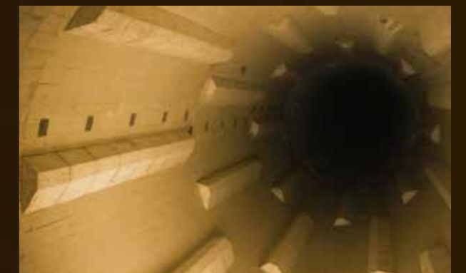
Special shape lifter blocks with stainless steel reinforced matrix and high temperature pre-firing.
