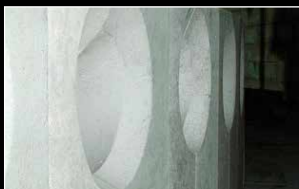
Pre-assembly of gas inlet nozzles, made out of special mullite/corundum material
