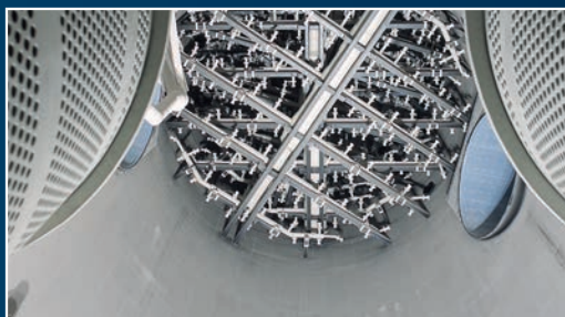
Flue gas desulphurization scrubber – Steuler rubber linings for very high chemical, thermal and mechanical requirements.
