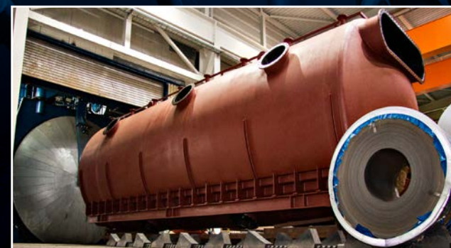
Rubber-lined steel tanks after vulcanisation in the autoclave.
