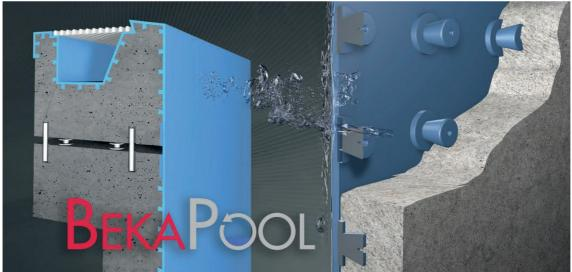
Prefabricated coping element with height-adjustable overflow channel (left) and system cross section of the composite materials. Credit: Steuler
